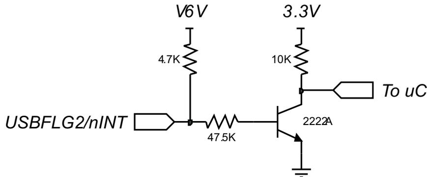
Figure 5. Circuit for Level-Shifting and Inverting nINT Signal
