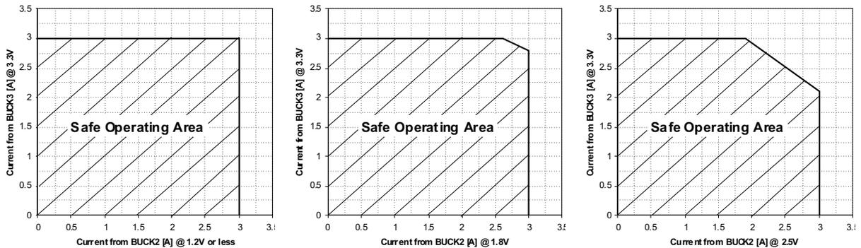
For any voltage / current combination inside the shaded area, the dissipated power inside the chip is below the allowable maximum. The examples assume  $T_{ambient} < 60^{\circ}C$ ,  $\eta = 90\%$  and  $\theta_{JA} < 44^{\circ}C/W$ .
