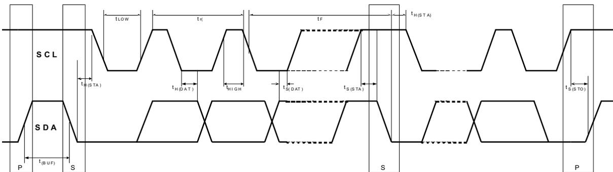
Figure 8. I<sup>2</sup>C Data Transmission Timing
