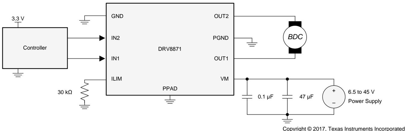
Figure 7. Typical Connections
