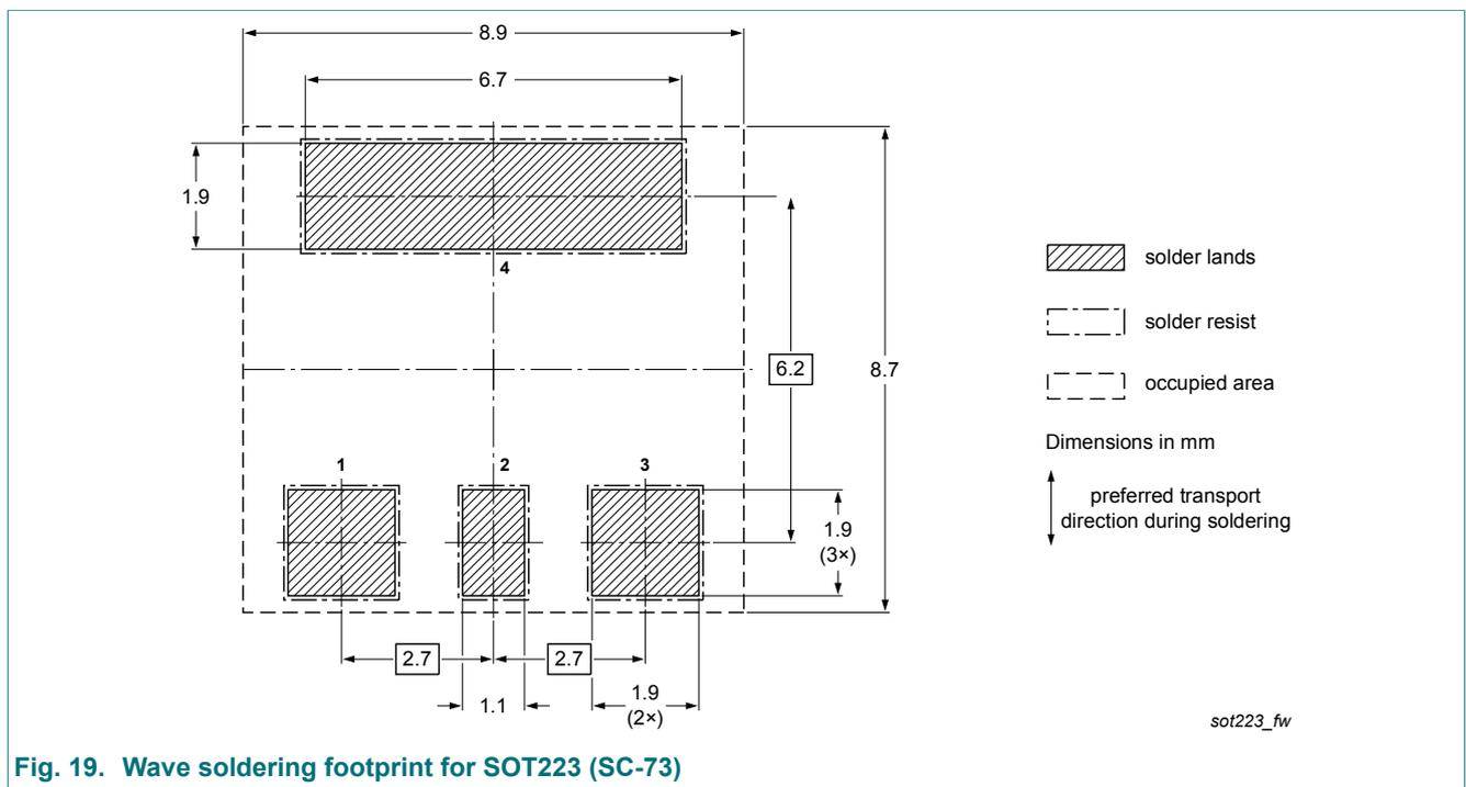
Fig. 19. Wave soldering footprint for SOT223 (SC-73)
