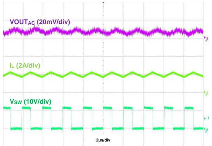
Figure 15. Output Voltage Ripple,  $V_{OUT} = 5\text{V}$ ,  $I_{OUT} = 2\text{A}$
