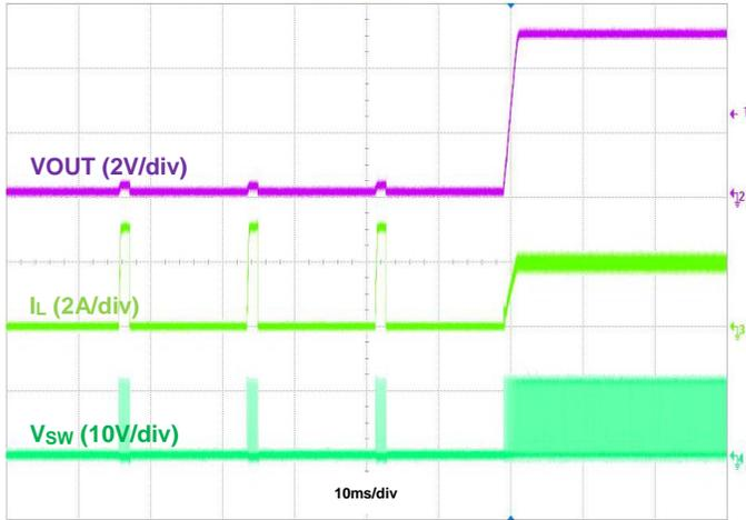
Figure 24. Output Short Recovery, IOU = 2A
