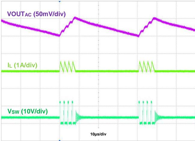
Figure 16. Output Voltage Ripple,  $V_{OUT} = 3.3\text{V}$ ,  $I_{OUT} = 50\text{mA}$
