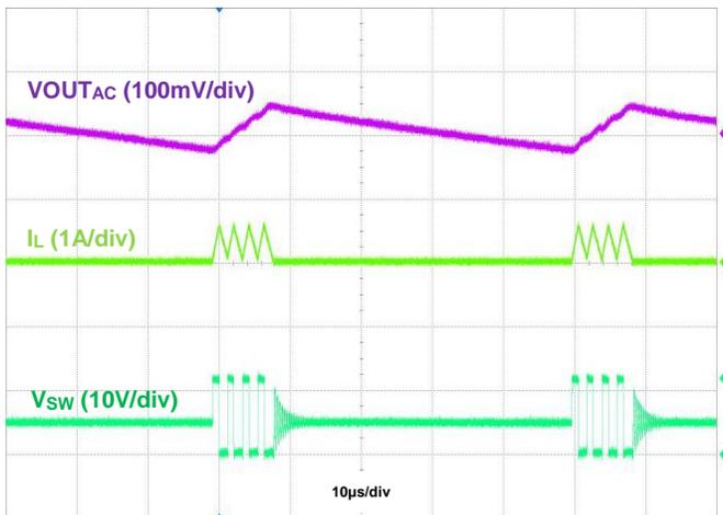
Figure 14. Output Voltage Ripple,  $V_{OUT} = 5\text{V}$ ,  $I_{OUT} = 50\text{mA}$
