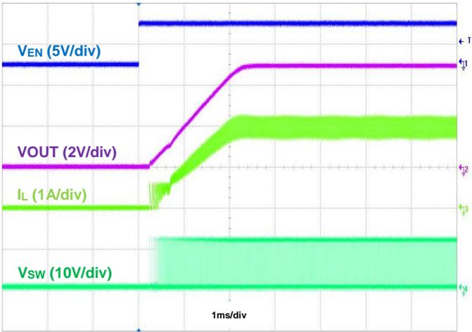
Figure 21. Startup Using EN, IOU = 2A
