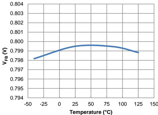
Figure 8. Feedback Voltage vs. Temperature,  $I_{OUT} = 1\text{A}$
