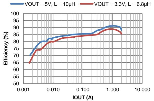
Figure 5. Efficiency vs. Output Current,  $V_{IN} = 24\text{V}$
