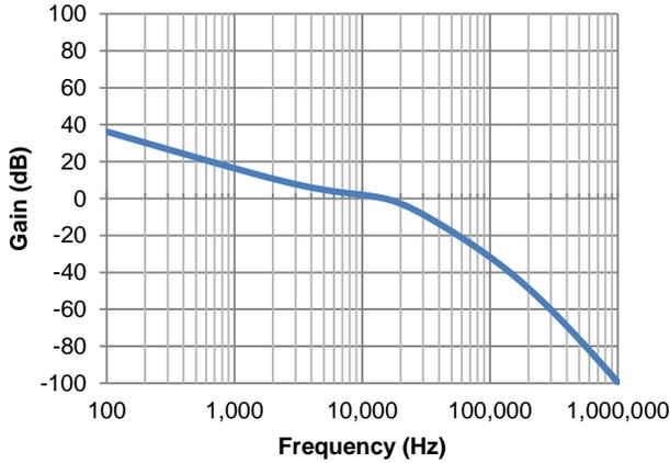
Figure 32. Closed-Loop Bandwidth
