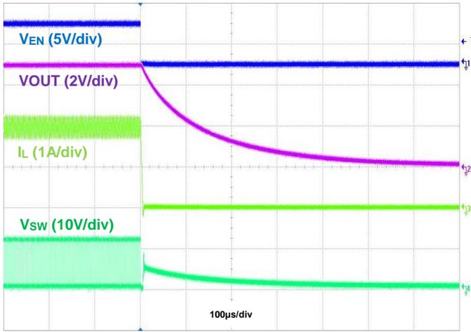
Figure 22. Shutdown Using EN, IOU = 2A
