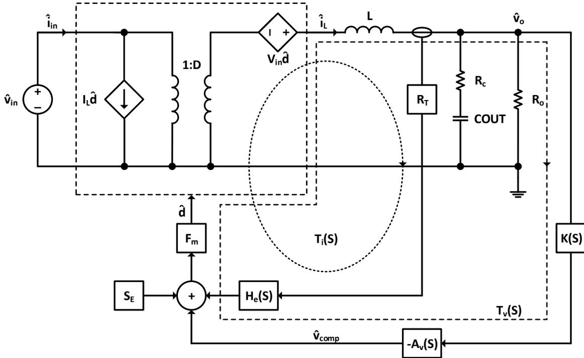
Figure 28. Small Signal Model of Buck Regulator
