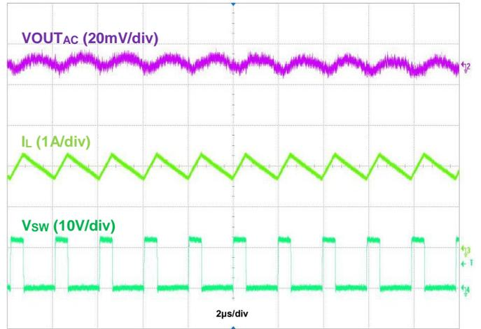
Figure 17. Output Voltage Ripple,  $V_{OUT} = 3.3\text{V}$ ,  $I_{OUT} = 2\text{A}$
