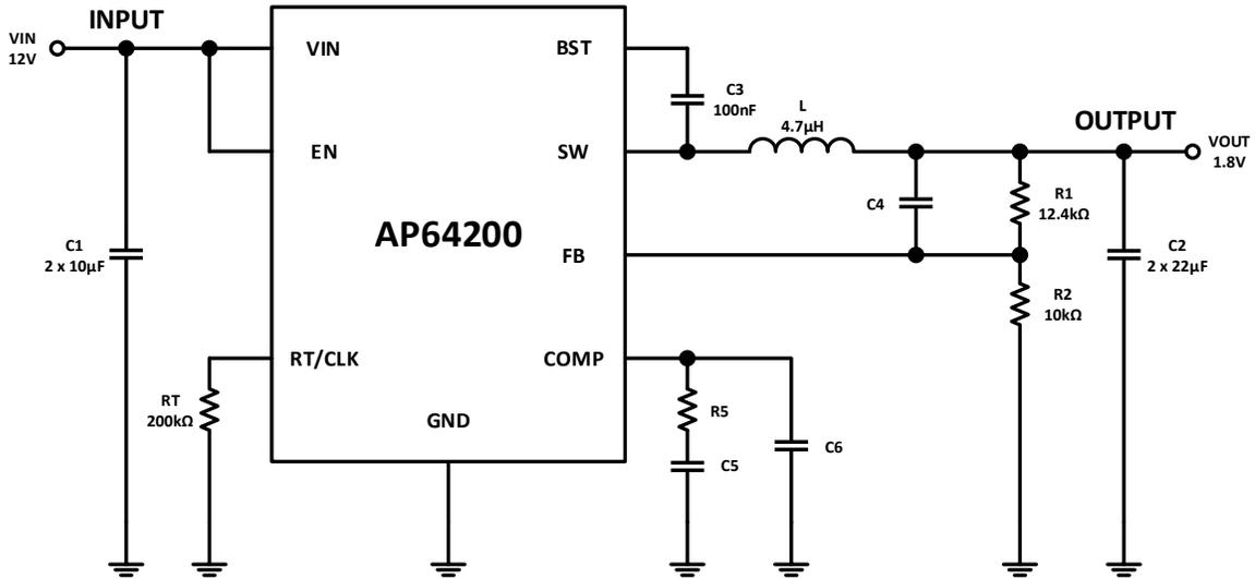
**Figure 30. Example Circuit for Loop Compensation Calculations**
