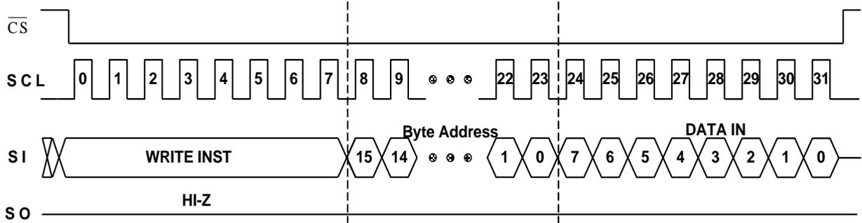
Figure 10: WRITE Timing
