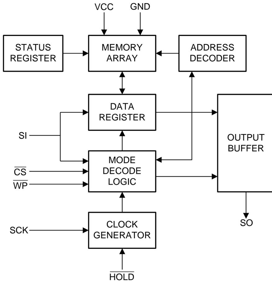
Figure 2: Block Diagram
