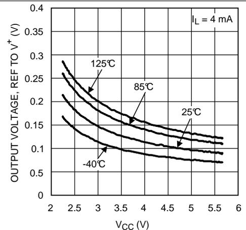
Figure 6. Output Voltage vs Supply Voltage
