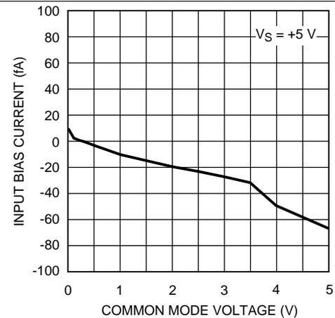
Figure 5. Input Bias vs Common Mode at 25°C
