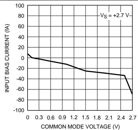
Figure 4. Input Bias vs Common Mode at 25°C
