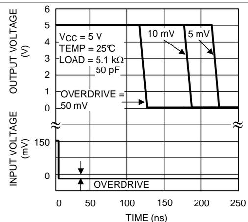
Figure 18. Response Time vs Input Overdrives Negative Transition
