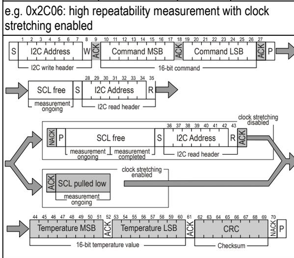
**Table 7** Measurement commands in single shot mode (Clear blocks are controlled by the microcontroller, grey blocks by the sensor)
