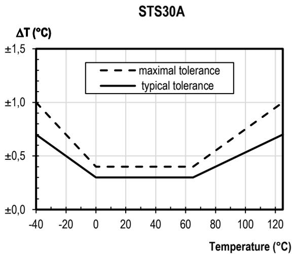
Figure 2 Temperature accuracy of the STS30A sensor.
