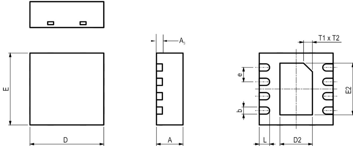
Figure 7 Dimensional drawing of STS3xA-DIS sensor package
