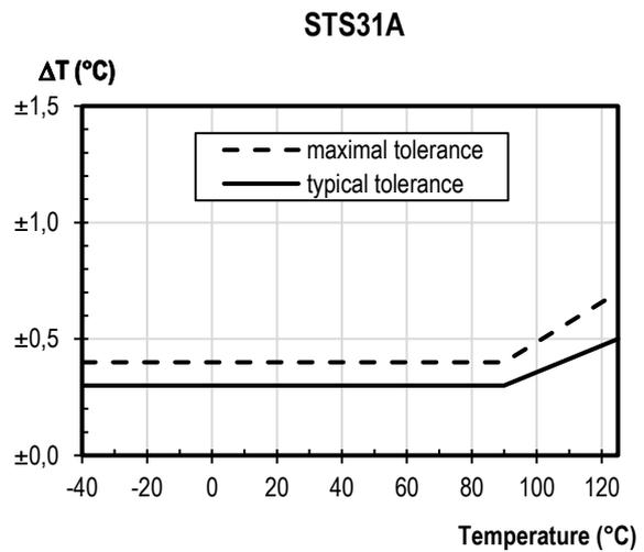
Figure 3 Temperature accuracy of the STS31A sensor.
