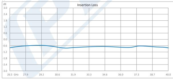
Click the following link (or enter part number in "SEARCH" on website) to obtain additional part information including price, inventory and certifications: Isolator with 12 dB Isolation from 26.5 GHz to 40 GHz, 10 Watts and 2.92mm Female to 2.92mm Male PE83IR1037
