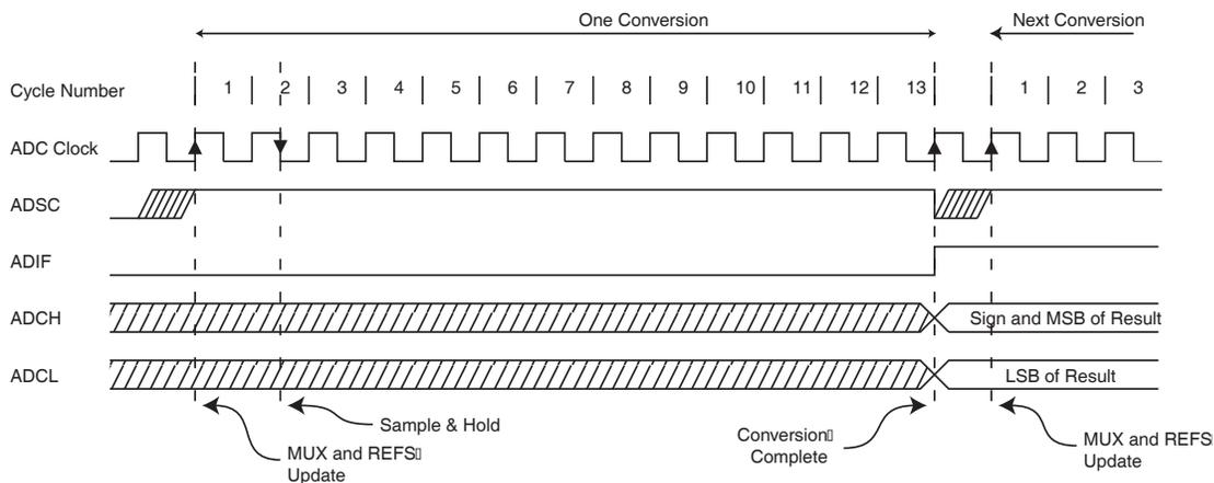
When Auto Triggering is used, the prescaler is reset when the trigger event occurs, as shown in [Figure 14-6](#) below. This assures a fixed delay from the trigger event to the start of conversion. In this mode, the sample-and-hold takes place two ADC clock cycles after the rising edge on the trigger source signal. Three additional CPU clock cycles are used for synchronization logic.
