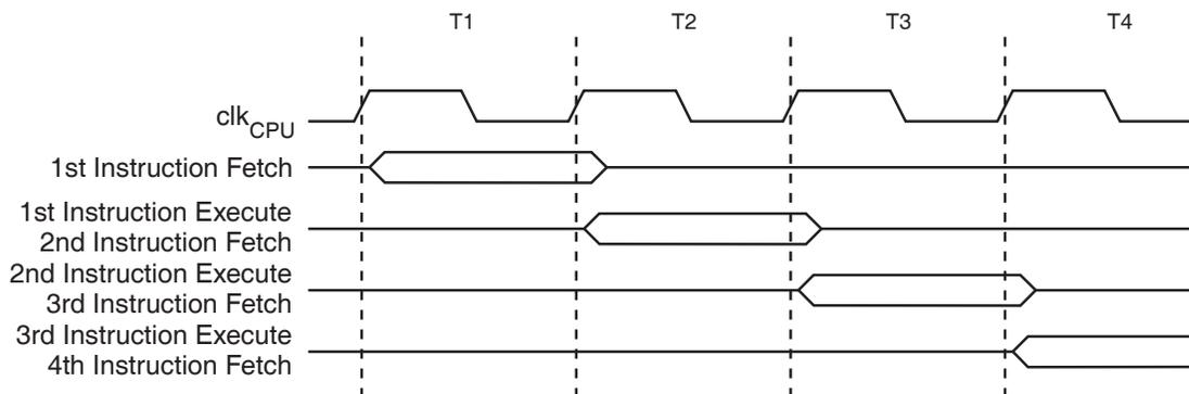
Figure 4-5 on page 18 shows the internal timing concept for the Register File. In a single clock cycle an ALU operation using two register operands is executed, and the result is stored back to the destination register.
