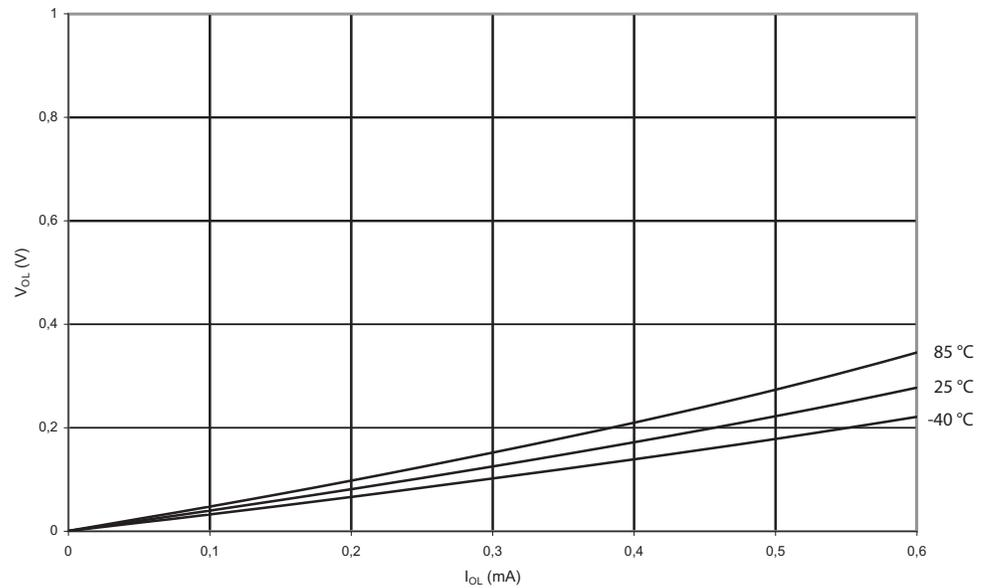
**Figure 19-43.**  $V_{OL}$ : Reset Pin as I/O, Output Voltage vs. Sink Current ( $V_{CC} = 3V$ )
