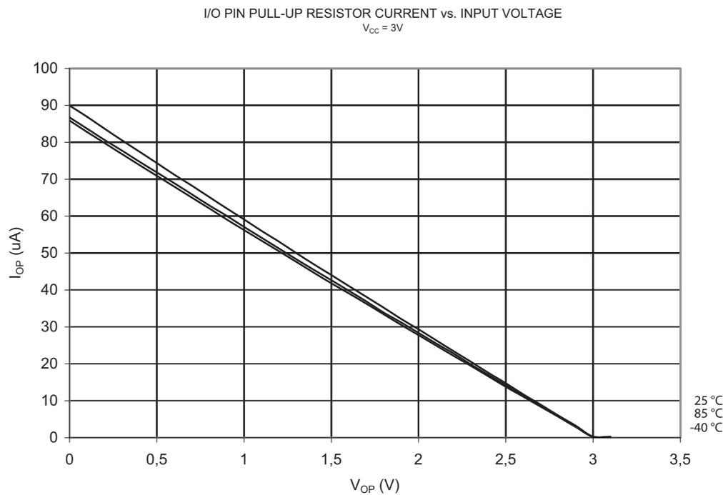
**Figure 19-23.** Pull-up Resistor Current vs. Input Voltage (I/O Pin,  $V_{CC} = 5V$ )
