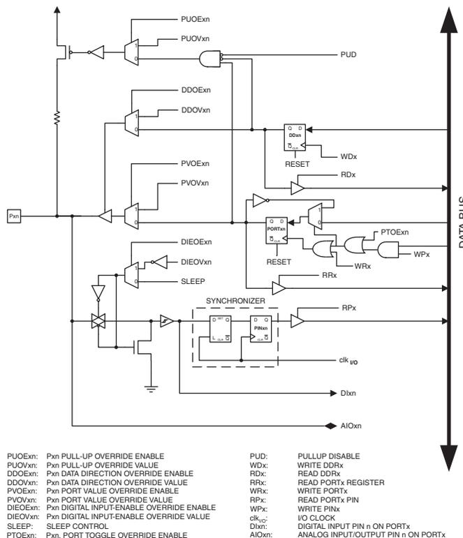
Note: WRx, WPx, WDx, RRx, RPx, and RDx are common to all pins within the same port. clk<sub>I/O</sub>, SLEEP, and PUD are common to all ports. All other signals are unique for each pin.
