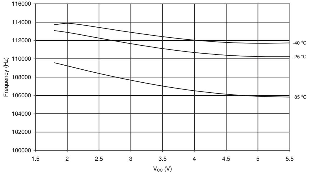
**Figure 19-66.** 128 kHz Watchdog Oscillator Frequency vs. Temperature
