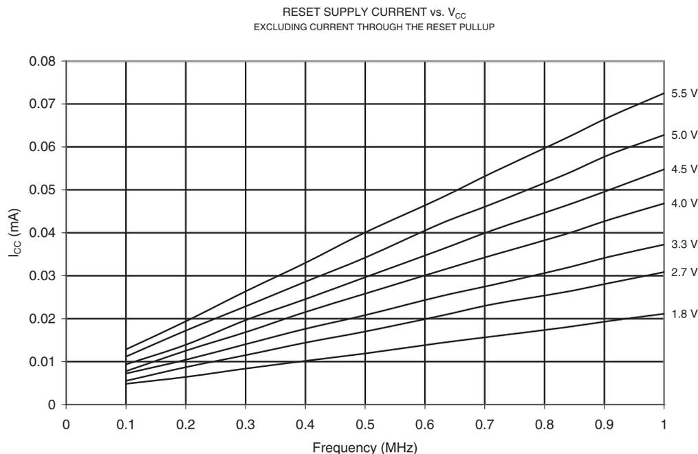
**Figure 19-16.** Reset Supply Current vs.  $V_{CC}$  (1 - 20 MHz, Excluding Current through the Reset Pull-up)
