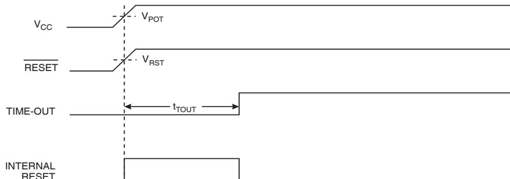
**Figure 8-3.** MCU Start-up,  $\overline{RESET}$  Extended Externally
