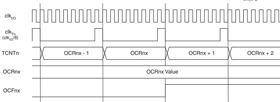
Figure 11-11 shows the setting of OCF0A and the clearing of TCNT0 in CTC mode and fast PWM mode where OCR0A is TOP.
