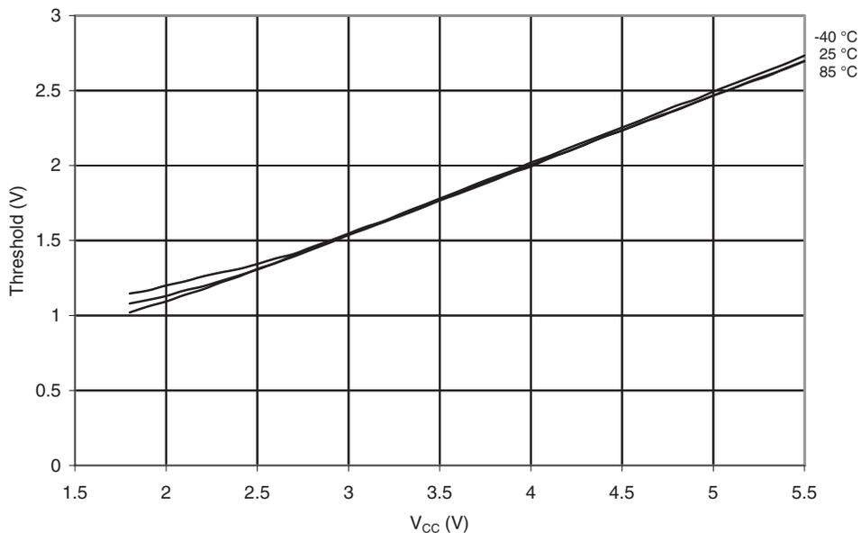
**Figure 19-49.**  $V_{IL}$ : Input Threshold Voltage vs.  $V_{CC}$  (Reset Pin as I/O, Read as '0')
