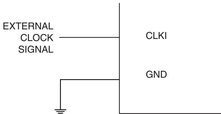
When this clock source is selected, start-up times are determined by the SUT fuses as shown in [Table 6-3](#).
