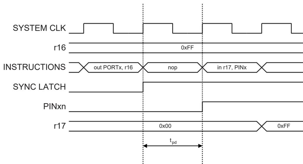
The following code example shows how to set port B pins 0 and 1 high, 2 and 3 low, and define the port pins from 4 to 5 as input with a pull-up assigned to port pin 4. The resulting pin values are read back again, but as previously discussed, a nop instruction is included to be able to read back the value recently assigned to some of the pins.
