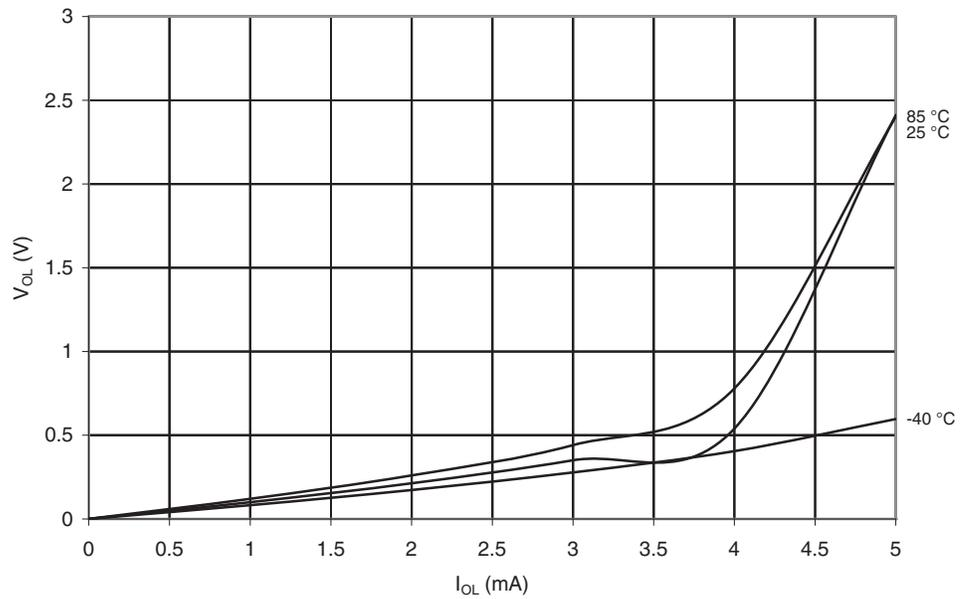
**Figure 19-31.**  $V_{OL}$ : I/O Pin Output Voltage vs. Sink Current (Low Power Pins,  $V_{CC} = 3V$ )
