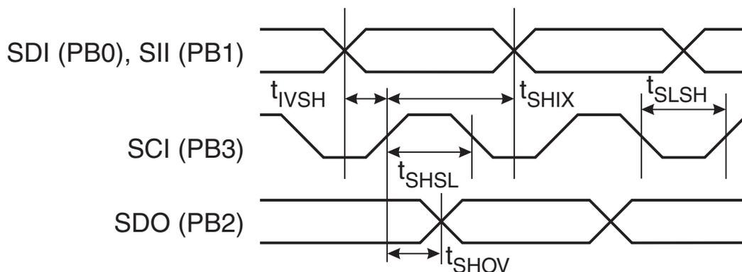
**Table 18-10.** High-voltage Serial Programming Characteristics
