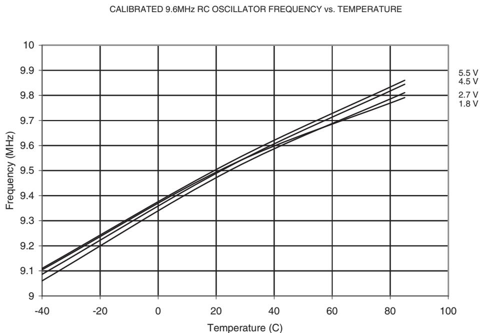
**Figure 19-60.** Calibrated 9.6 MHz RC Oscillator Frequency vs.  $V_{CC}$
