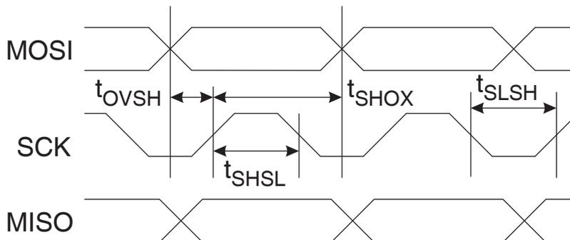
**Figure 18-4.** Serial Programming Waveform
