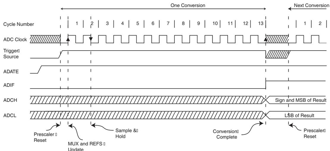
In Free Running mode, a new conversion will be started immediately after the conversion completes, while ADSC remains high.
