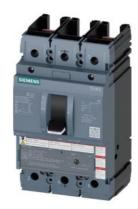
circuit breaker 3VA5 UL frame 250 breaking capacity class C 100kA @ 480V 2-pole, line protection TM230, FTAM, In=200A overload protection Ir=200A fixed short-circuit protection Ii=5...10 x In without connection
