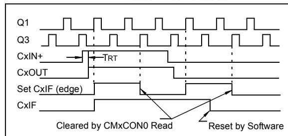
**Note 1:** If a change in the CMxCON0 register (CxOUT) should occur when a read operation is being executed (start of the Q2 cycle), then the CxIF interrupt flag of the PIR2 register may not get set.
