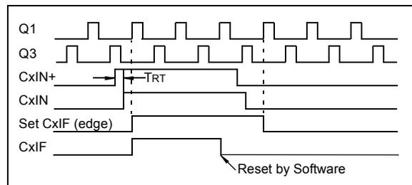
**FIGURE 19-4: COMPARATOR INTERRUPT TIMING WITH CMxCON0 READ**
