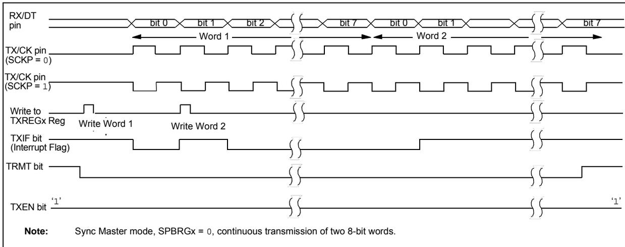
**FIGURE 17-11: SYNCHRONOUS TRANSMISSION (THROUGH TXEN)**
