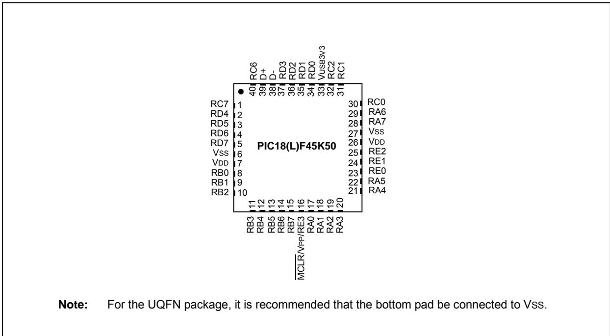
**Note:** For the UQFN package, it is recommended that the bottom pad be connected to VSS.
