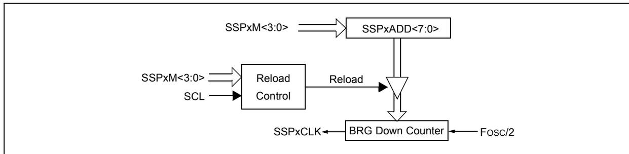
**Note:** Values of 0x00, 0x01 and 0x02 are not valid for SSPxADD when used as a Baud Rate Generator for I<sup>2</sup>C™. This is an implementation limitation.
