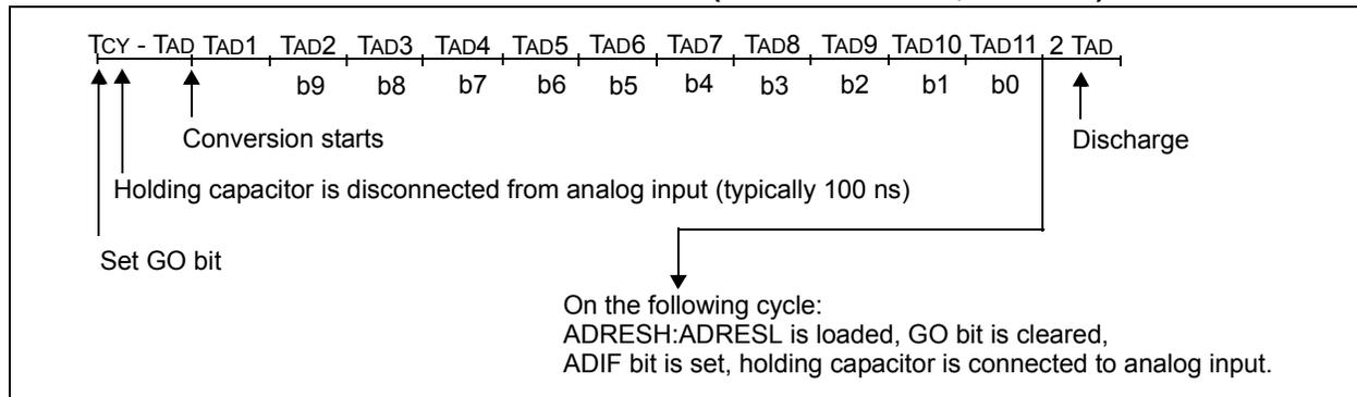
**FIGURE 18-4: A/D CONVERSION TAD CYCLES (ACQT<2:0> = 010, TACQ = 4 TAD)**
