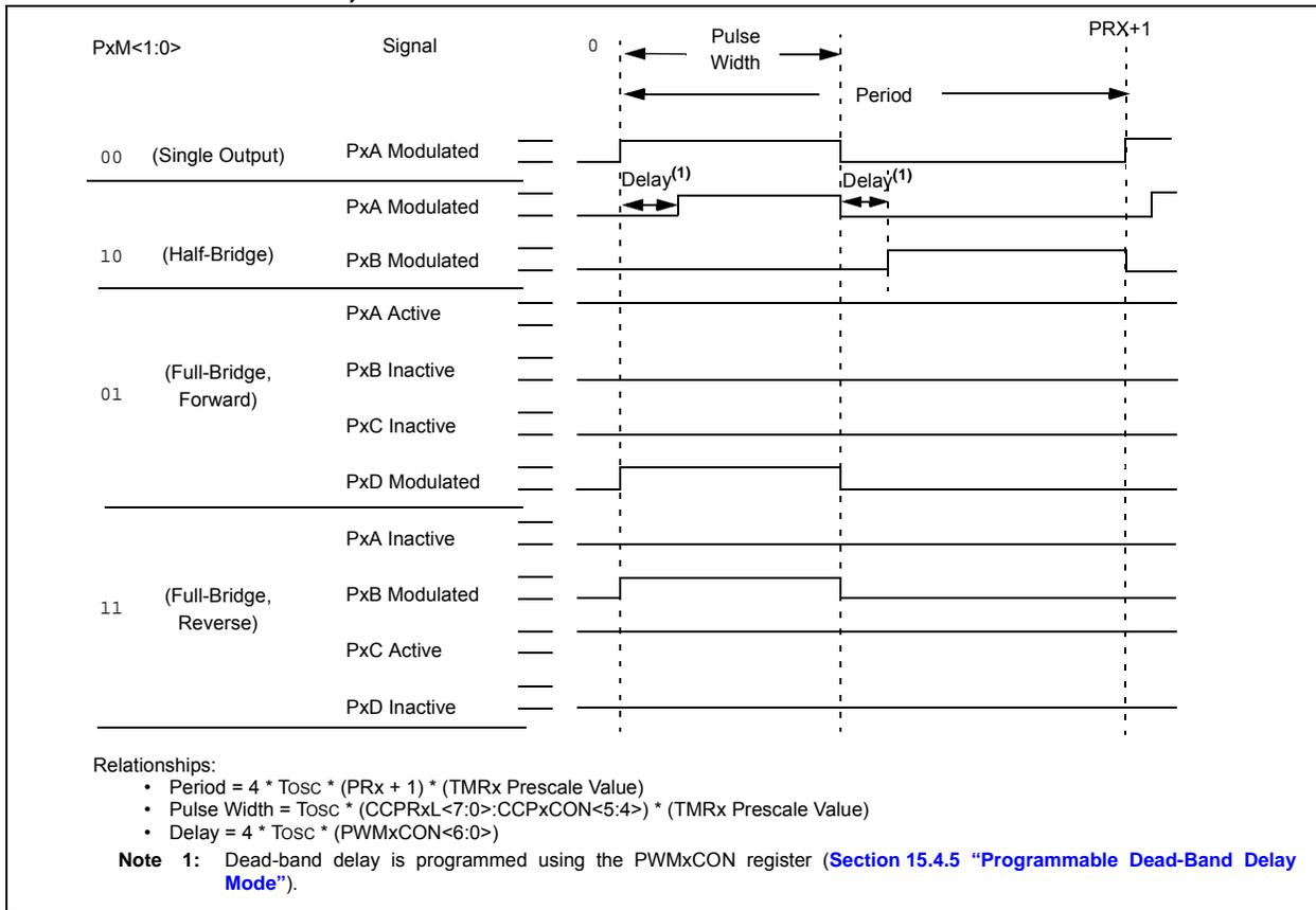
**FIGURE 15-7: EXAMPLE ENHANCED PWM OUTPUT RELATIONSHIPS (ACTIVE-LOW STATE)**
