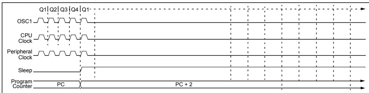
**FIGURE 4-5: TRANSITION TIMING FOR WAKE FROM SLEEP (HSPLL)**
