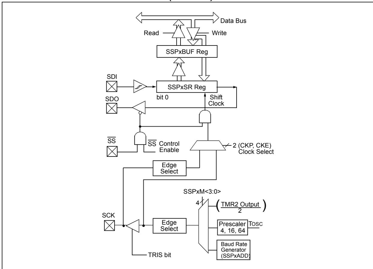
**FIGURE 16-3: MSSP BLOCK DIAGRAM (I<sup>2</sup>C™ SLAVE MODE)**
