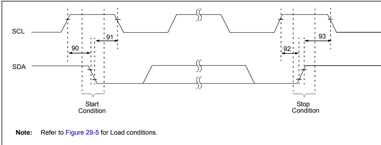
**TABLE 29-28: MASTER SSP I<sup>2</sup>C™ BUS START/STOP BITS REQUIREMENTS**
