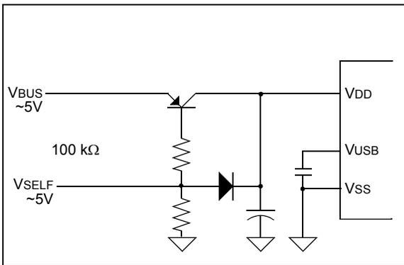
**Note:** Users should keep in mind the limits for devices drawing power from the USB. According to USB Specification 2.0, this cannot exceed 100 mA per low-power device or 500 mA per high-power device.
