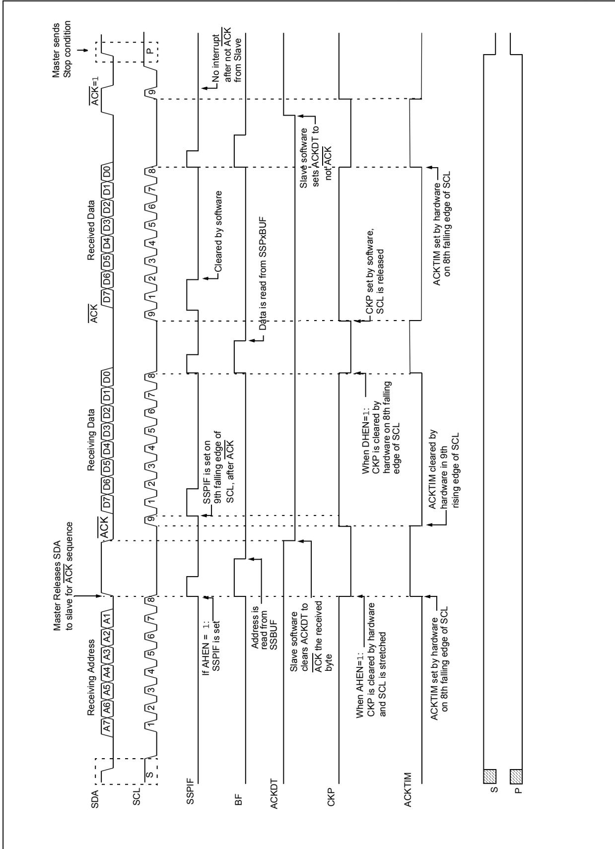
FIGURE 16-17: I<sup>2</sup>C™ SLAVE, 7-BIT ADDRESS, RECEPTION (SEN = 1, AHEN = 1, DHEN = 1)
