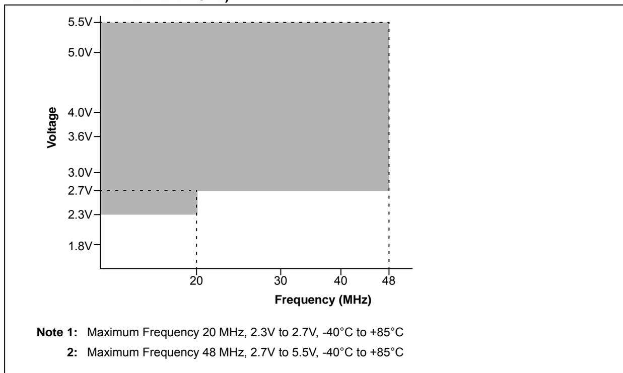
**FIGURE 29-3: PIC18F2X/45K50 FAMILY VOLTAGE-FREQUENCY GRAPH (EXTENDED TEMPERATURE)**
