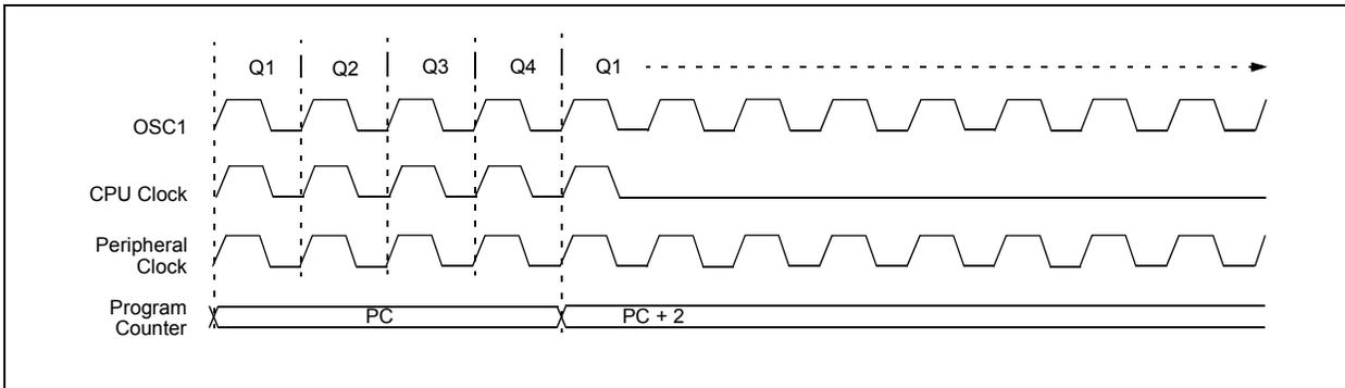
**FIGURE 4-7: TRANSITION TIMING FOR WAKE FROM IDLE TO RUN MODE**
