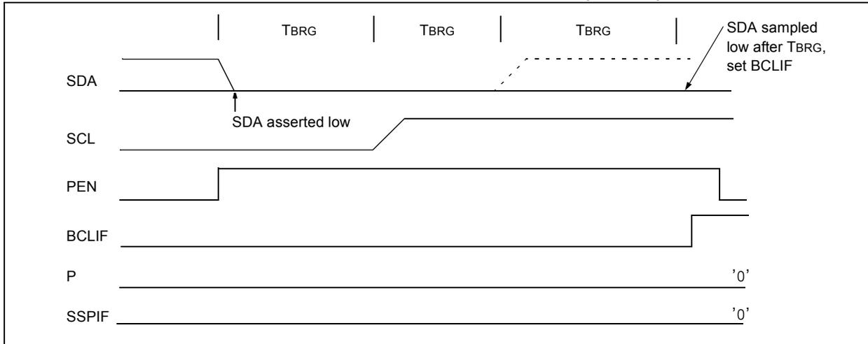
**FIGURE 16-39: BUS COLLISION DURING A STOP CONDITION (CASE 2)**
