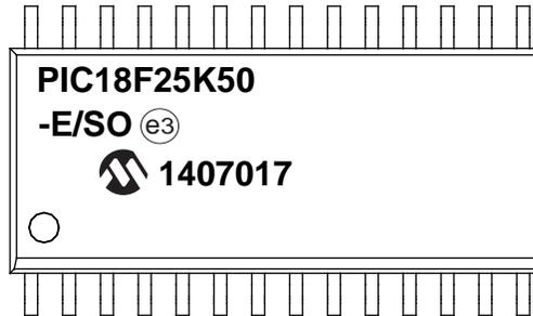
28-Lead SSOP (5.30 mm)
