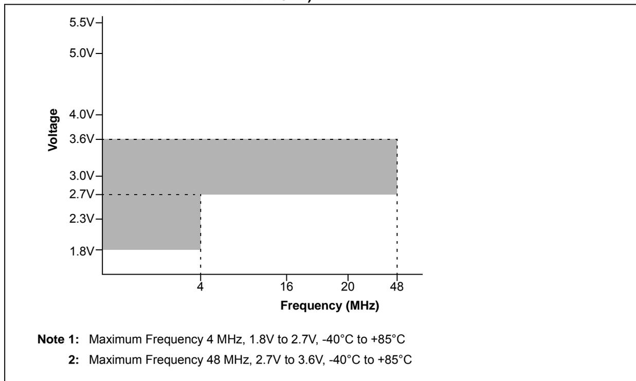
**FIGURE 29-2: PIC18F2X/45K50 FAMILY VOLTAGE-FREQUENCY GRAPH (INDUSTRIAL TEMPERATURE)**
