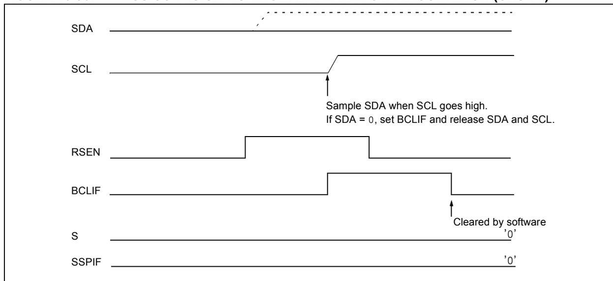
**FIGURE 16-37: BUS COLLISION DURING REPEATED START CONDITION (CASE 2)**
