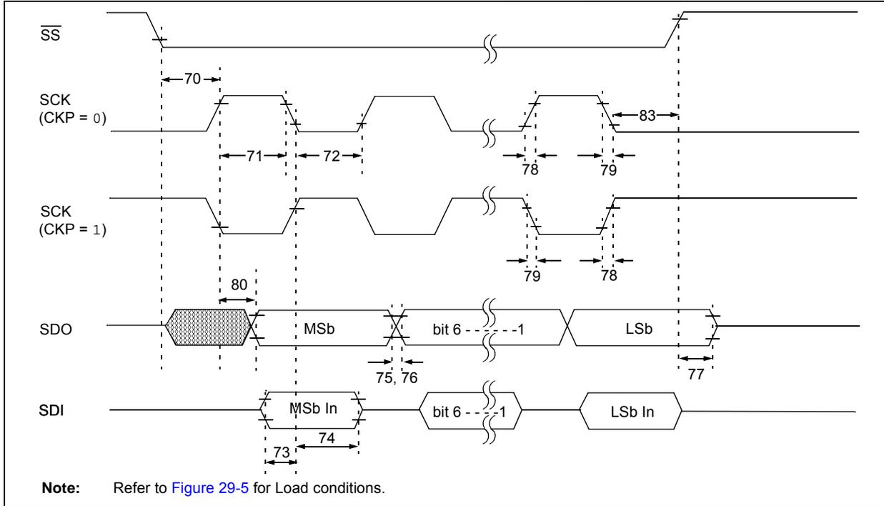
**TABLE 29-25: EXAMPLE SPI MODE REQUIREMENTS (SLAVE MODE TIMING, CKE = 0 OR 1)**
