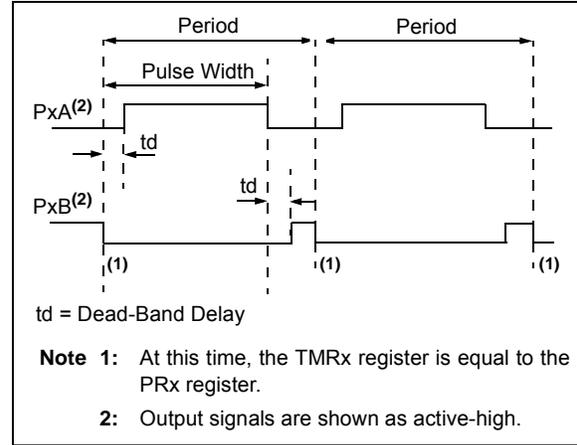
**FIGURE 15-9: EXAMPLE OF HALF-BRIDGE APPLICATIONS**
