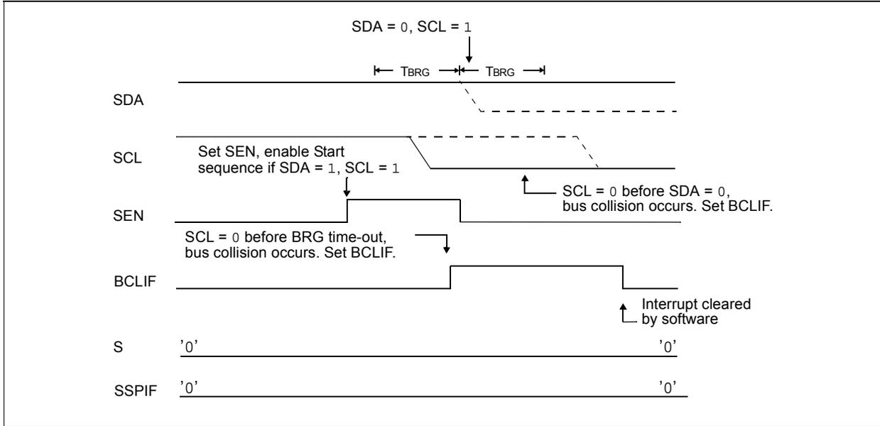
**FIGURE 16-35: BRG RESET DUE TO SDA ARBITRATION DURING START CONDITION**
