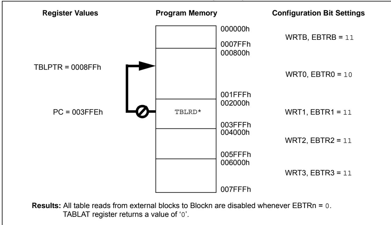
**FIGURE 26-5: INTERNAL BLOCK TABLE READ (EBTRn) ALLOWED**
