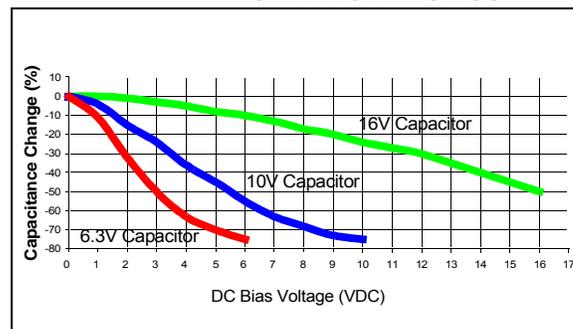
When selecting a ceramic capacitor to be used with the internal voltage regulator, it is suggested to select a high-voltage rating, so that the operating voltage is a small percentage of the maximum rated capacitor voltage. For example, choose a ceramic capacitor rated at 16V for the 3.3V VUSB3V3 voltage.
