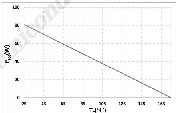
Fig. 4 Typical Power Derating
