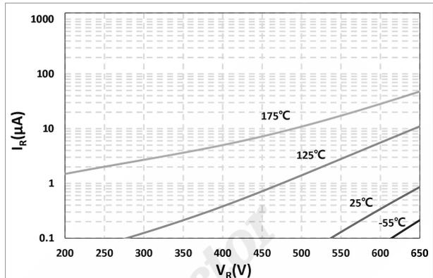
Fig. 2 Reverse Characteristics
