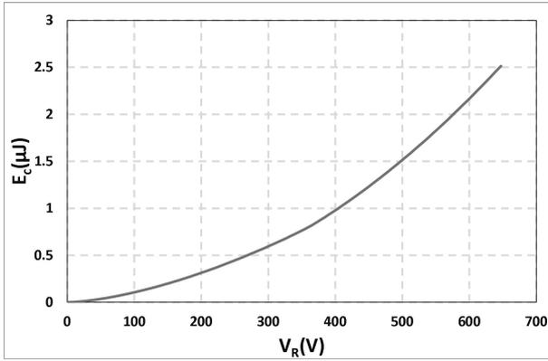
Fig. 7 Capacitance Stored Energy
