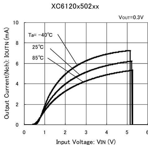
(5) Output Current (Pch Driver) vs. Input Voltage
