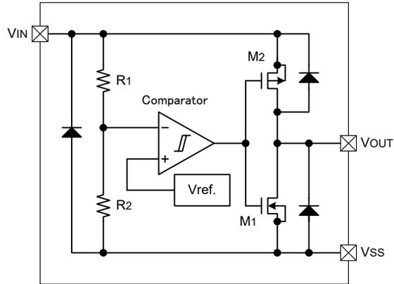
\* Diodes inside the circuits are ESD protection diodes and parasitic diodes.
