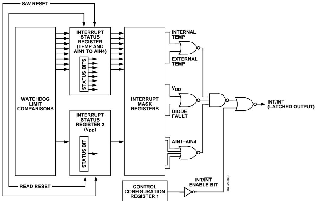
Figure 49. Interrupt Structure
