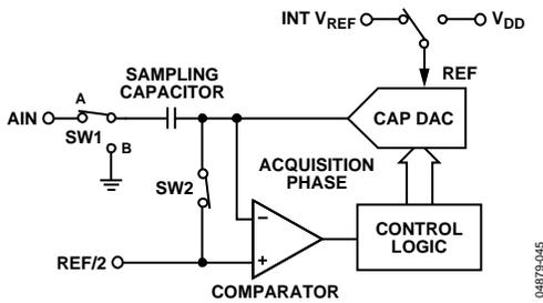
Figure 45. ADC Acquisition Phase
