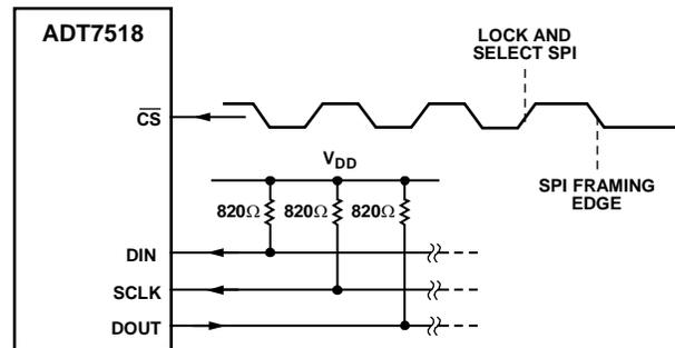
Figure 55. Typical SPI Interface Connection
