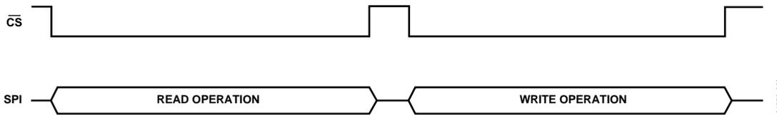
Figure 63. SPI—Correct Use of  $\overline{CS}$  During SPI Communication
