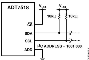
Figure 54. Typical I<sup>2</sup>C Interface Connection
