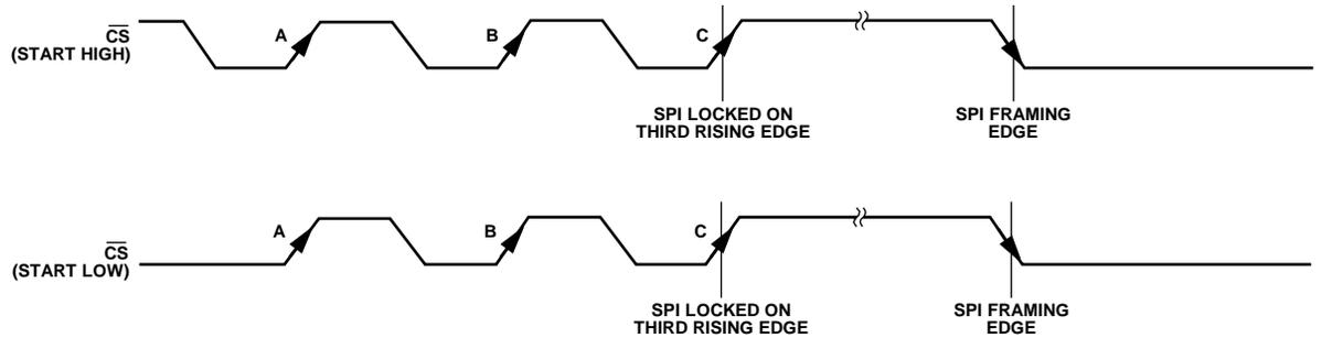
Figure 53. Serial Interface—Selecting and Locking SPI Protocol
