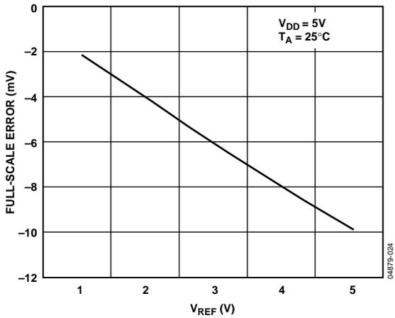
Figure 24. DAC Full-Scale Error vs. V<sub>REF</sub>
