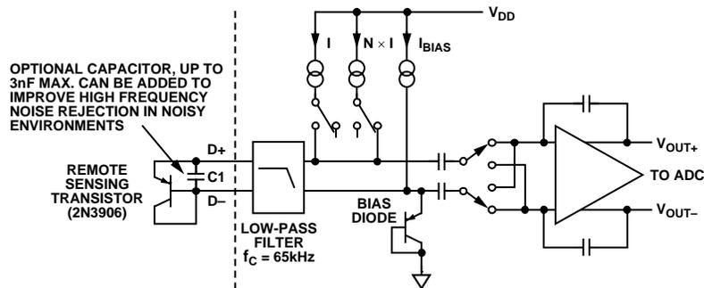
Figure 41. Signal Conditioning for External Diode Temperature Sensor
