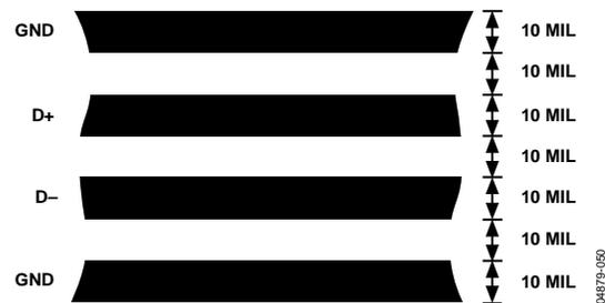
Figure 50. Arrangement of Signal Tracks
