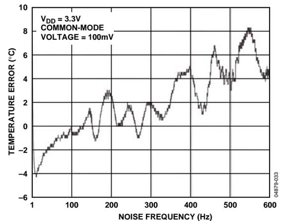
Figure 33. External Temperature Error vs. Common-Mode Noise Frequency
