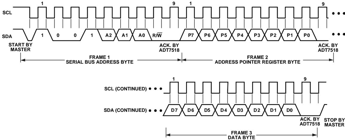
Figure 57. I<sup>2</sup>C—Writing to the Address Pointer Register Followed by a Single Byte of Data to the Selected Register
