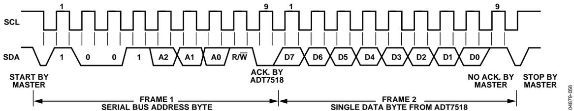
Figure 58. I<sup>2</sup>C—Reading a Single Byte of Data from a Selected Register
