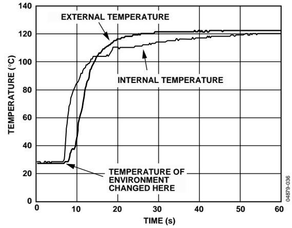
Figure 36. Temperature Sensor Response to Thermal Shock
