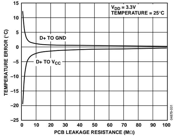
Figure 31. External Temperature Error vs. PCB Leakage Resistance
