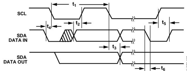
Figure 2. I<sup>2</sup>C Bus Timing Diagram
