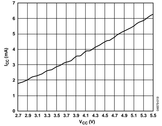
Figure 19. Power-Down Current vs. Supply Voltage @ 25°C
