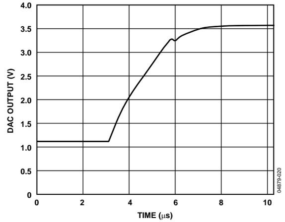
Figure 20. DAC Half-Scale Settling (1/4 to 3/4 Scale Code Change)
