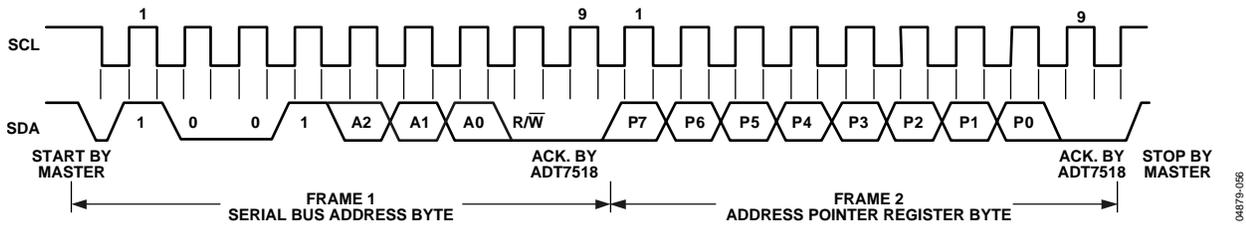
Figure 56. I<sup>2</sup>C—Writing to the Address Pointer Register to Select a Register for a Subsequent Read Operation
