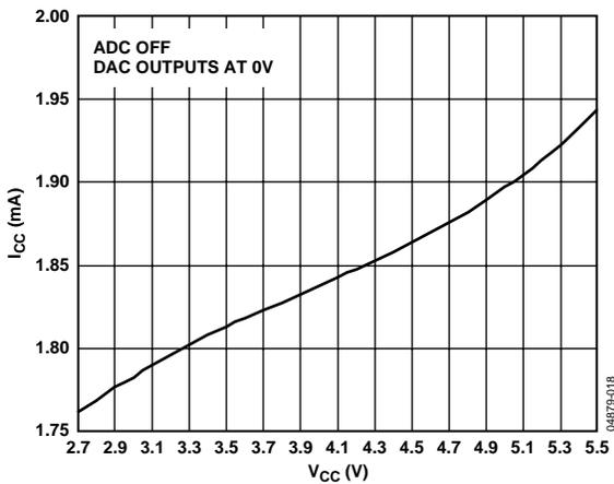
Figure 18. Supply Current vs. Supply Voltage @ 25°C
