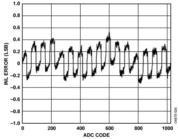
Figure 26. ADC INL with Ref = V<sub>DD</sub> (3.3 V)
