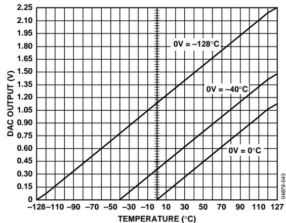
Figure 43. DAC Output vs. Temperature V<sub>REF-IN</sub> = 2.25 V
