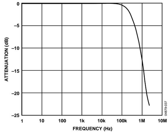
Figure 37. DAC Multiplying Bandwidth (Small Signal Frequency Response)
