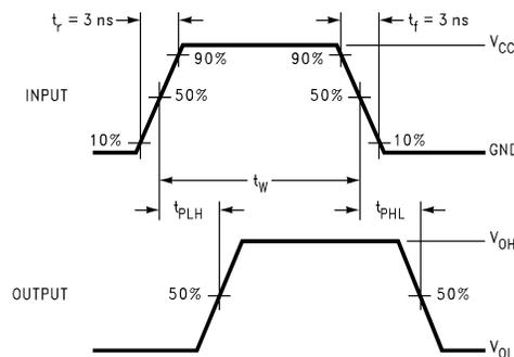
Figure 5. AC Waveforms
