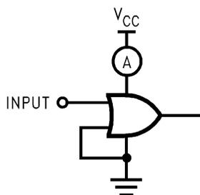
Figure 6. I<sub>CCD</sub> Test Circuit
