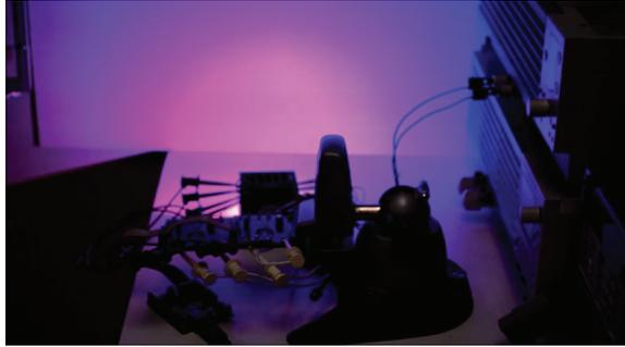
Figure 14. Complete digital control over high power RGBW LEDs using the LT3964 dual buck driver with I<sup>2</sup>C serial communications. Two LT3964s are enough to drive a single RGBW LED—or string of RGBW LEDs—at 1 A with accurate and precise dimming to produce predictably repeatable color content.
