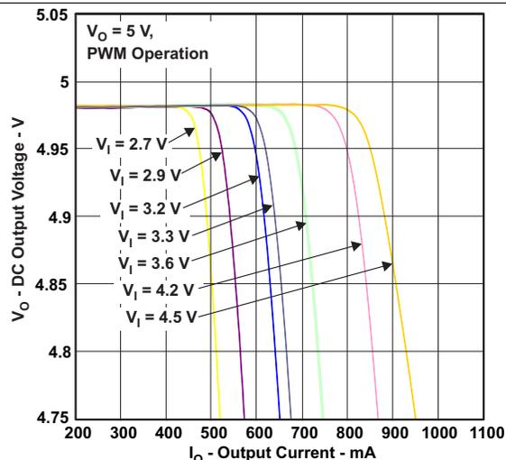
Figure 6. DC Output Voltage vs Output Current
