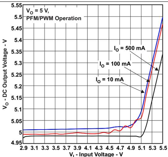
Figure 7. DC Output Voltage vs Input Voltage
