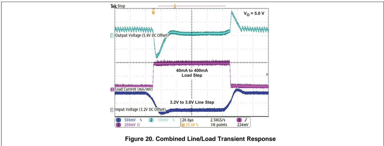
Figure 20. Combined Line/Load Transient Response
