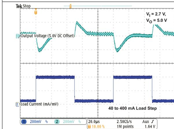
Figure 18. Load Transient Response In PFM/PWM Operation
