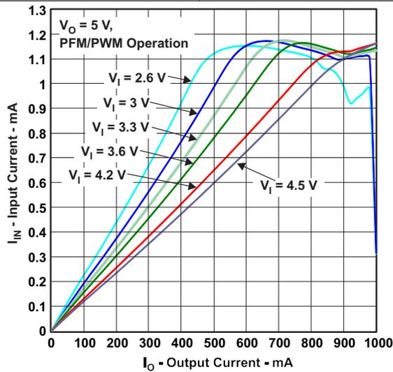
Figure 11. Input Current vs Output Current
