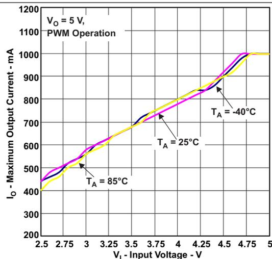
Figure 8. Maximum Output Current vs Input Voltage
