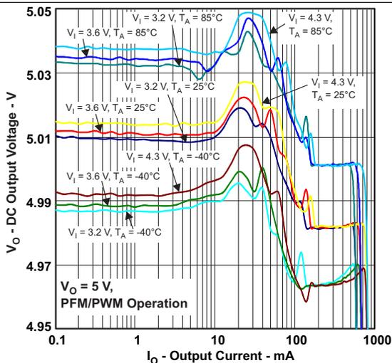
Figure 5. DC Output Voltage vs Output Current
