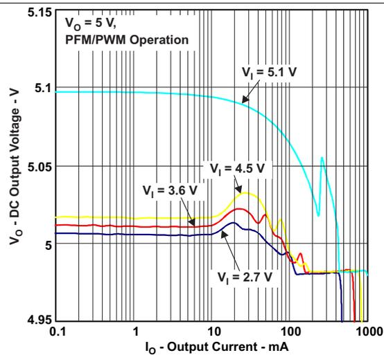
Figure 4. DC Output Voltage vs Output Current
