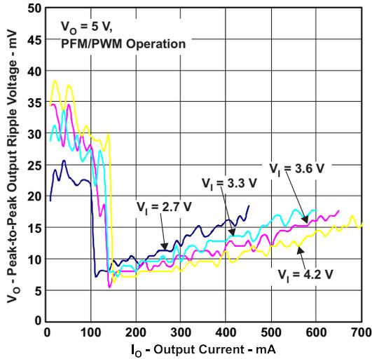
Figure 9. Peak-To-Peak Output Ripple Voltage vs Output Current
