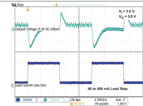
Figure 17. Load Transient Response In PFM/PWM Operation
