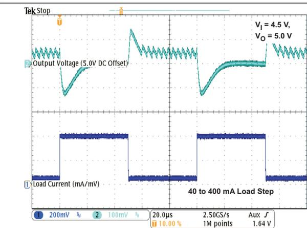
Figure 19. Load Transient Response In PFM/PWM Operation
