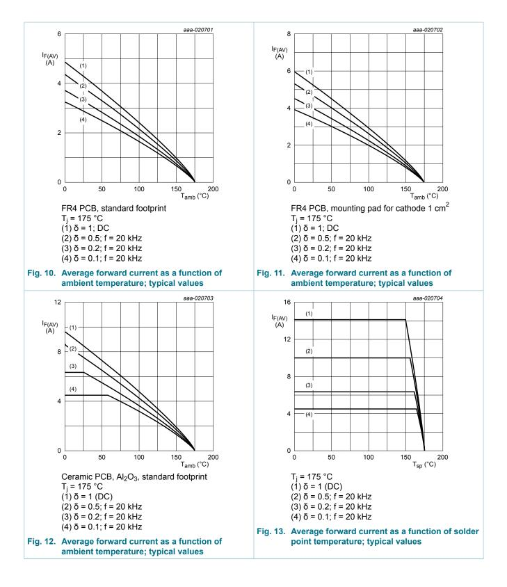
100 V, 10 A low leakage current Schottky barrier rectifier
