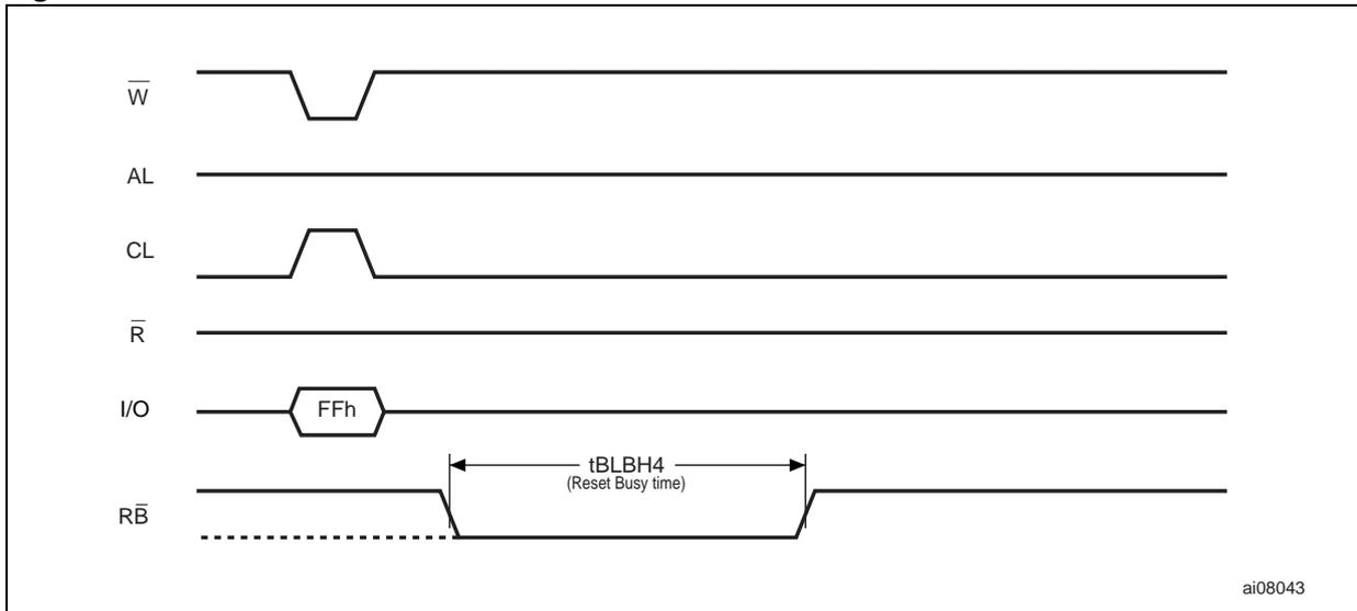
Figure 37. Program/erase enable waveform
