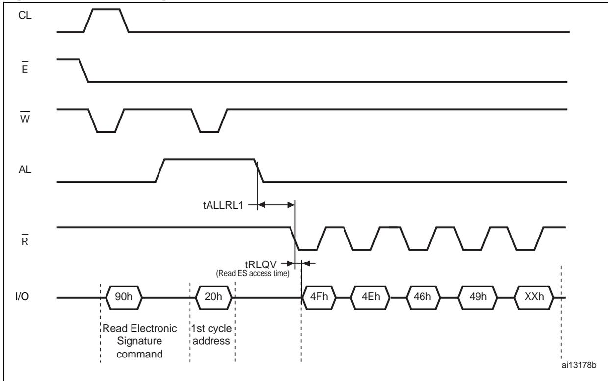
Figure 33. Page read operation AC waveform
