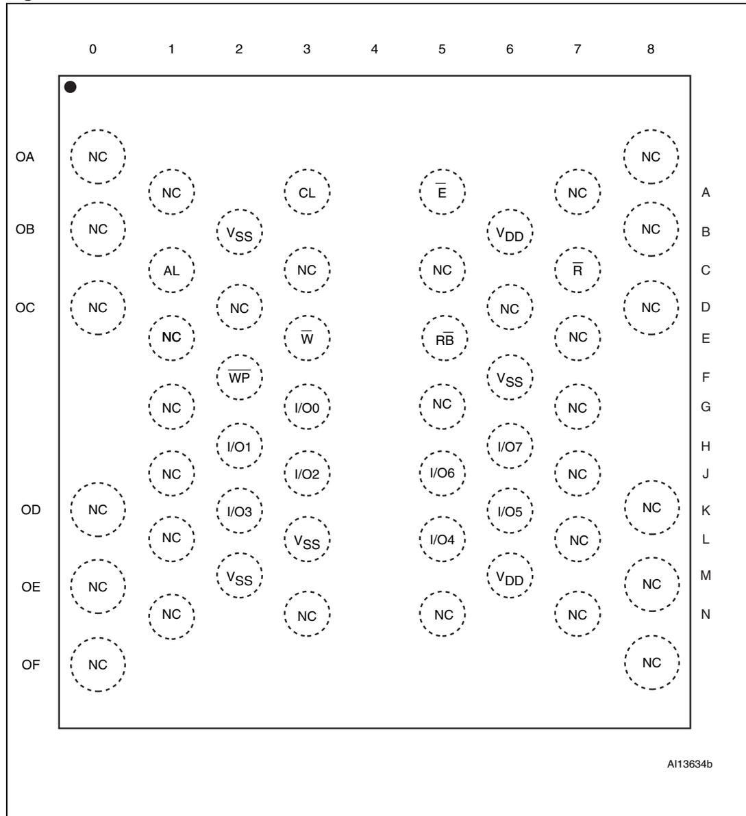
Figure 5. ULGA52 connections for the NAND08G-B4C devices
