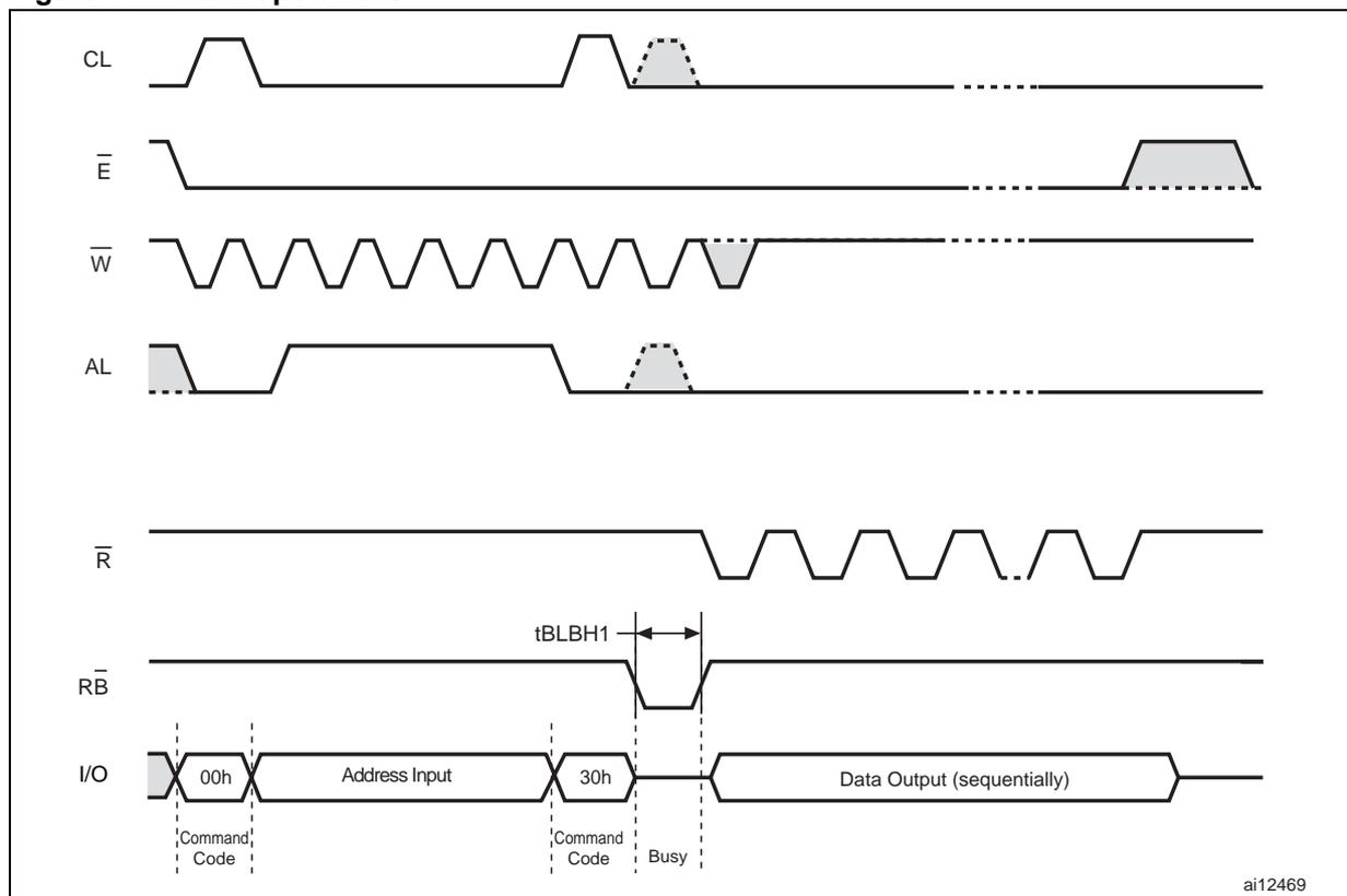
Figure 8. Random data output during sequential data output
