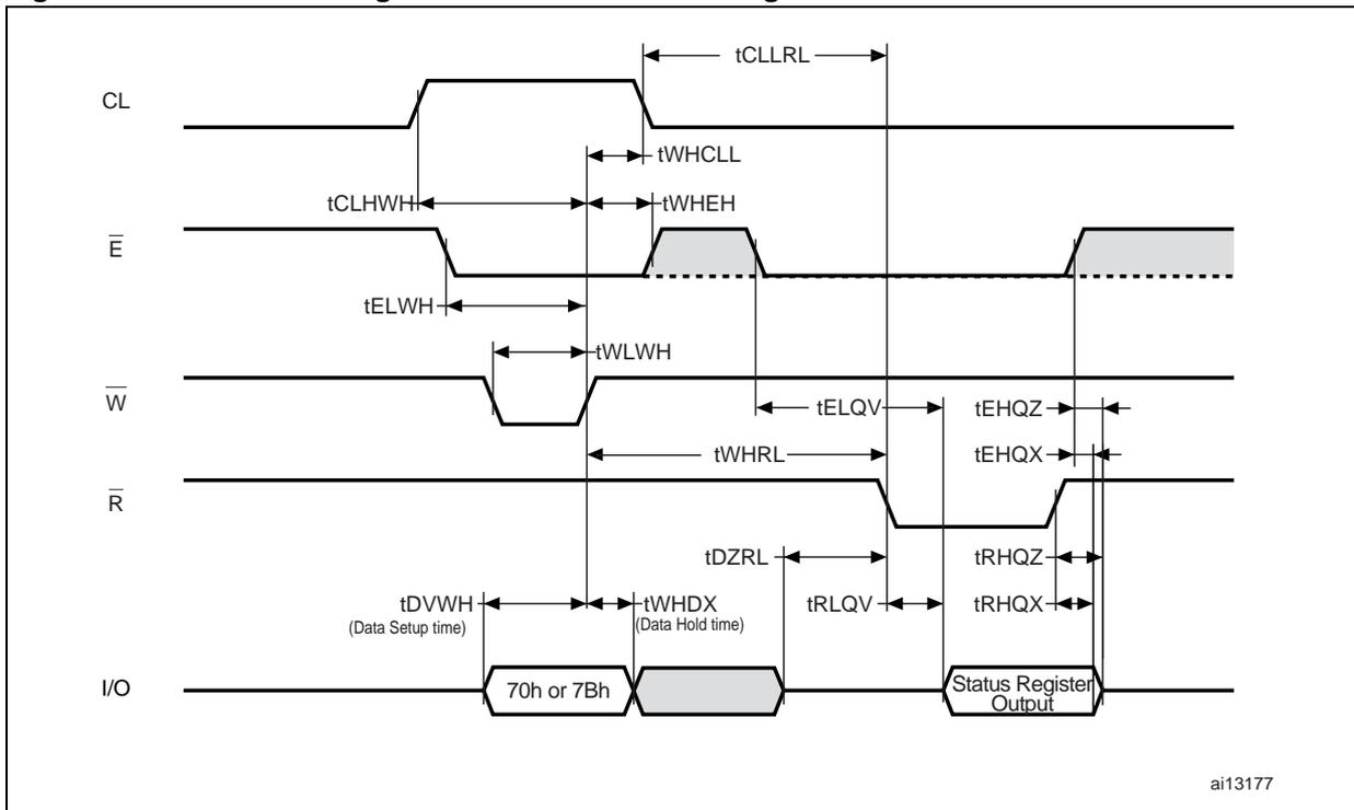
Figure 30. Read status enhanced waveform
