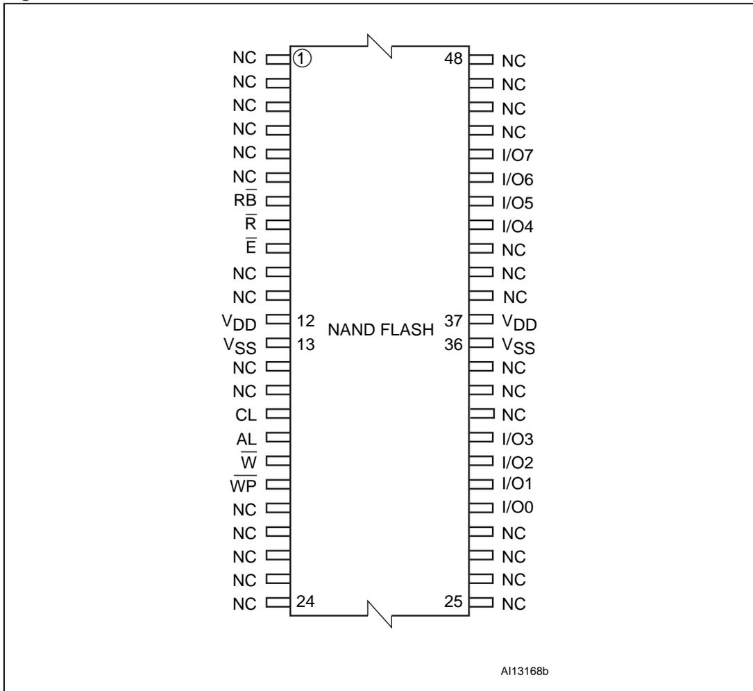
Figure 4. ULGA52 connections for NAND04G-B2D and NAND08G-B2C devices
