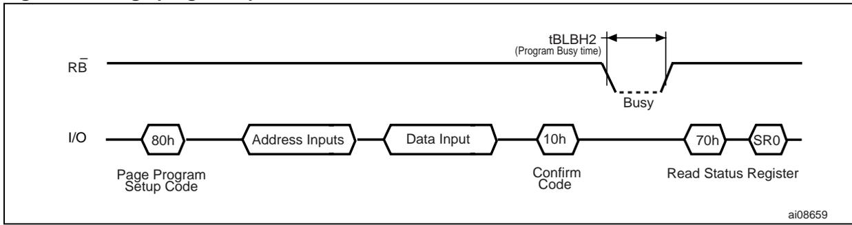
Figure 12. Random data input during sequential data input
