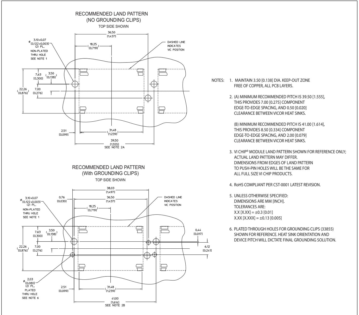
Figure 25 — Recommended heat sink push pin location
