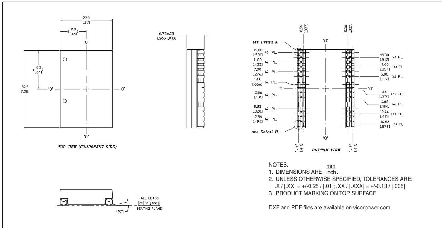
Figure 21 — PRM™ module J-Lead mechanical outline
