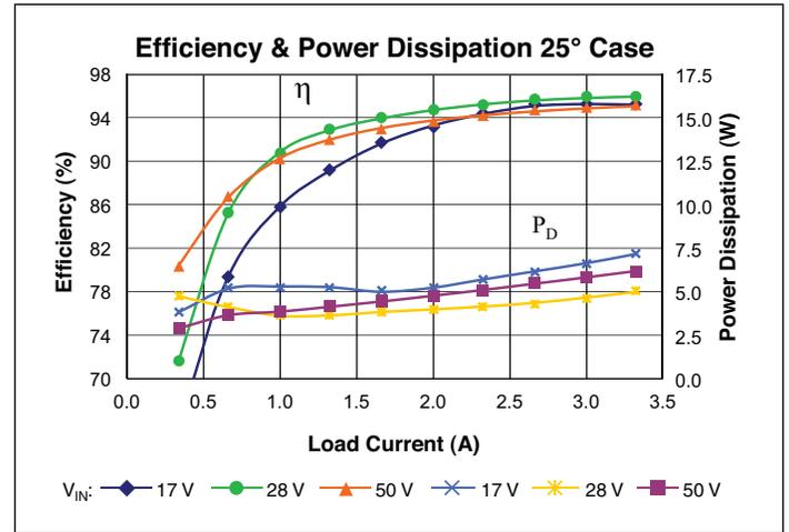
Figure 7 — Efficiency and power dissipation vs. output current at 36 V<sub>OUT</sub>, 25 °C T<sub>CASE</sub>
