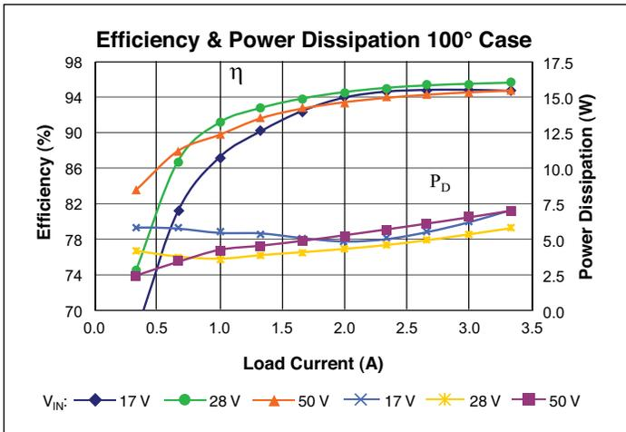
Figure 8 — Efficiency and power dissipation vs. output current at 36 V<sub>OUT</sub>, 100 °C T<sub>CASE</sub>
