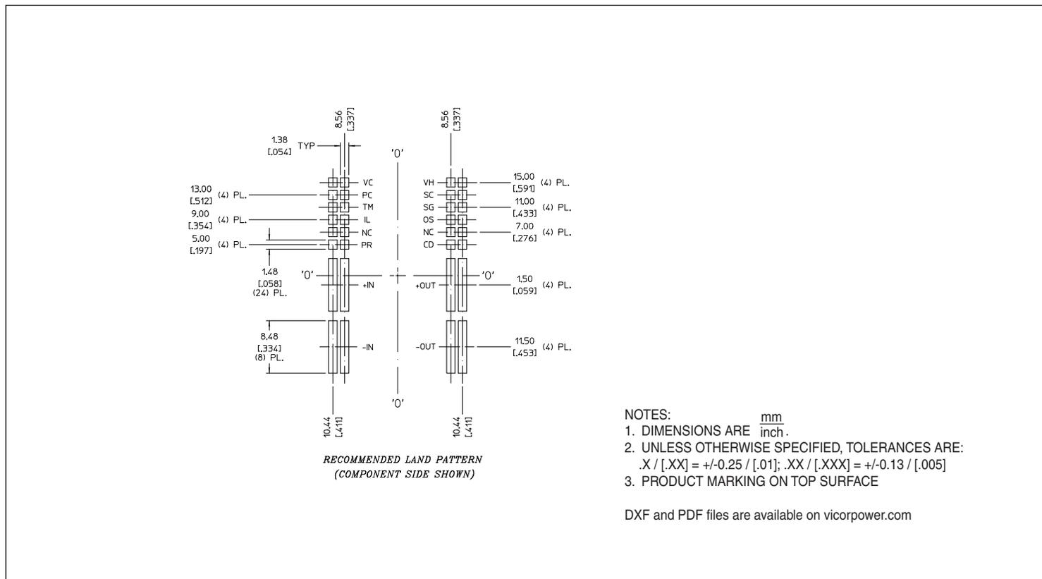
Figure 22 — PRM™ module J-Lead PCB land layout information
