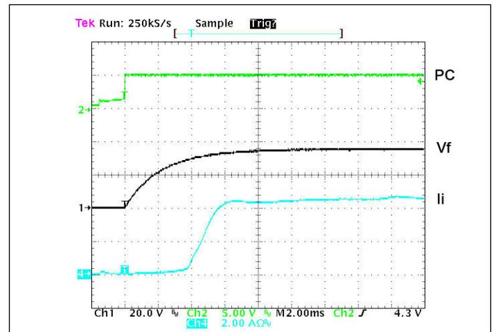
Figure 3 — V<sub>OUT</sub> turn on waveform with inrush current – PC enabled at full load, 28 V<sub>IN</sub>, electronic load set @ constant R.
