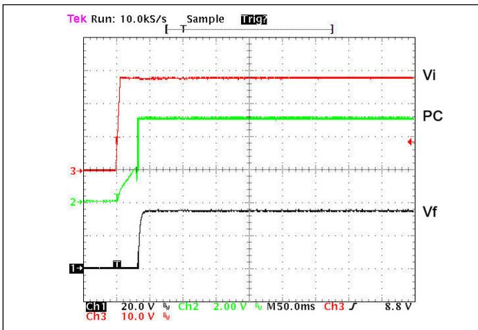
Figure 2 — V<sub>OUT</sub> and PC response from power up
