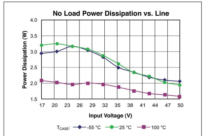
Figure 9 — No load power, unit enabled vs. line
