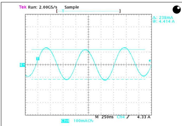
Figure 4 — Input reflected ripple current at full load and 28 V<sub>IN</sub>
