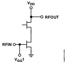
Figure 38. Basic Schematic for the Cascode Cell
