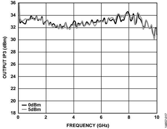
Figure 18. Output IP3 vs. Frequency for Various P<sub>OUT</sub>/Tone
