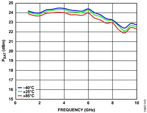
Figure 13.  $P_{SAT}$  vs. Frequency for Various Temperatures
