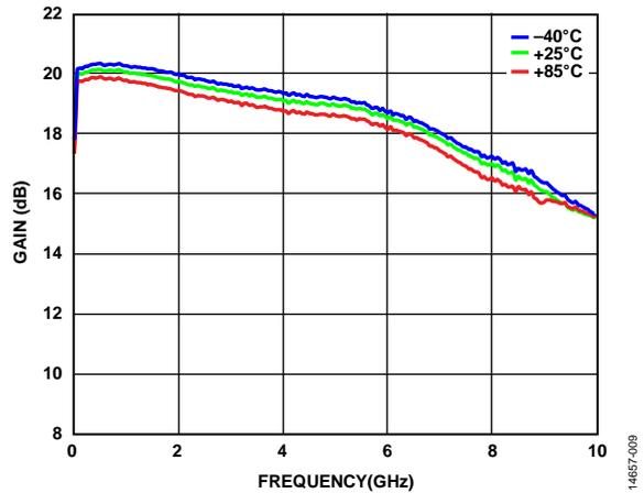
Figure 9. Gain vs. Frequency for Various Temperatures
