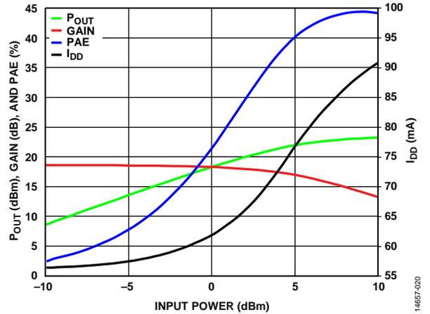
Figure 21. P<sub>OUT</sub>, Gain, PAE, and Supply Current with RF Applied (I<sub>DD</sub>) vs. Input Power at 5 GHz
