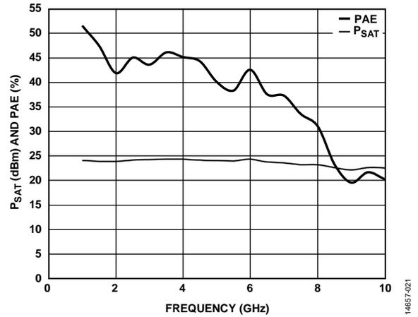
Figure 22. P<sub>SAT</sub> and PAE vs. Frequency
