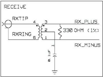
Figure 4. The original termination network for DS3150DK.
