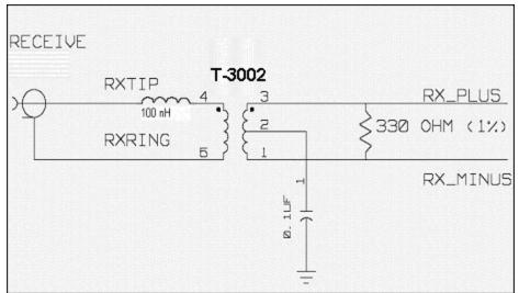
Figure 7. The modified termination network for the DS3150DK.
