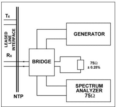
Figure 1. Return-loss measurement setup.
