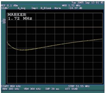
Figure 8. Return loss of the DS3150DK with modified termination network at 1720kHz.
