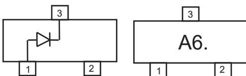
**350mW 100Volt Switching Diode**
