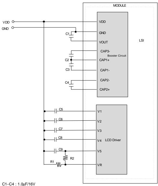
C1~C4:  $1.0\mu 1710V$ C5~C8:  $0.68\mu F/16V$ R1:  $270K\Omega \pm 0.2\%$ R2:  $1.1M\Omega \pm 0.2\%$
