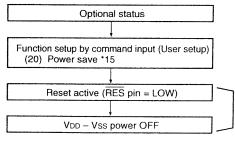
Set the time (t) from reset active to turning off the VDD - Vss power (VDD - Vss = 1.8 V) longer than the time ( $t_H$ ) when the potential of  $V_5 \sim V_1$ becomes below the threshold voltage (approximately 1 V) of the LCD panel. For th, refer to the <Reference Data> of this event. When  $t_H$  is too long, insert a resistor between  $V_5$  and  $V_{DD}$  to reduce it.
