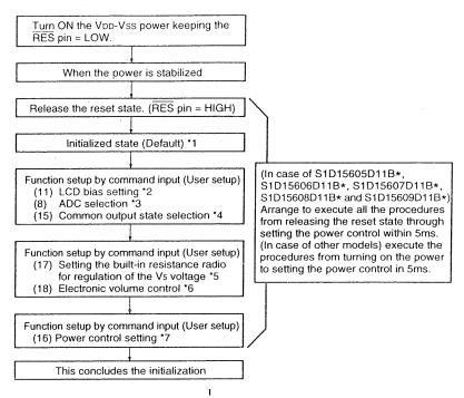
② When the built-in power is not being used immediately after turning on the power:
