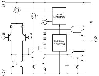
FIGURE 1. Equivalent schematic (one channel)
