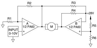
FIGURE 2. Bi-directional speed control from a single supply
